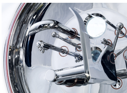
Scraper knife over the entire basket height, feed and wash pipe
