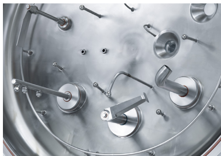
Feed and wash pipe, cake loosening device
