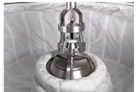
Filter bag with lifting device
