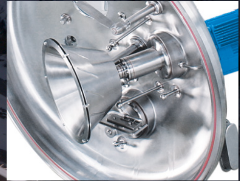
Inclined feed and wash disk, scraper knife with vertical movement
