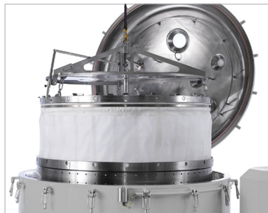
Lifting device for filter bag
